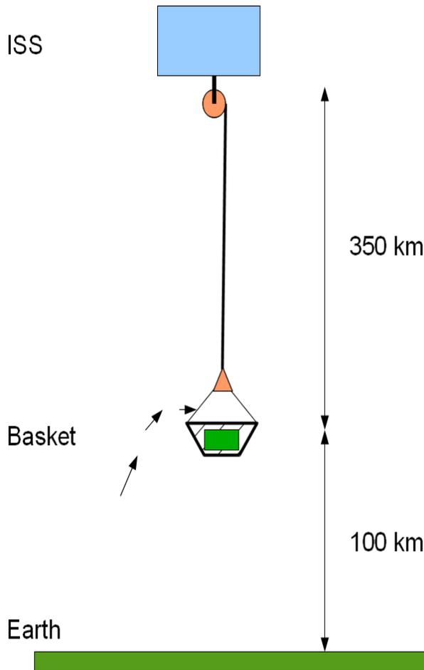
A calculation was conducted for the ISS at an altitude of 450 km, which is near the top of the normal operating range, as shown in Fig. 9. A tether was assumed to extend to an altitude of 100 km, below which heating may be a problem. The reduction in velocity requirement for transportation from Earth to ISS was reduced by 800 m/s.
