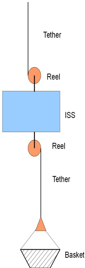
The next step will be addition of an exploration tether that extends from ISS to higher altitudes. It will also be a reel-tether. It will improve transportation from ISS to exploration destinations. The length of the exploration tether will also not be decided in this paper. The exploration tether would likely be much longer than the ISS tether, on the order of thousands of km.
